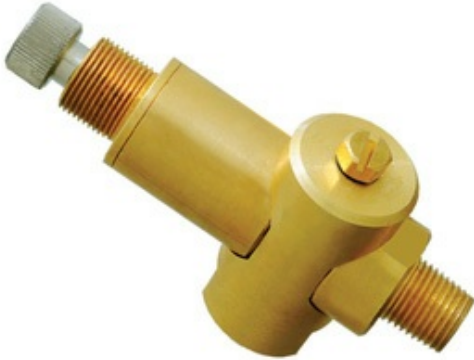
Pressure Regulator, 1/8" NPT Swivel Mount, Knurled Knob, Non-Relieving, 10-70 psig
