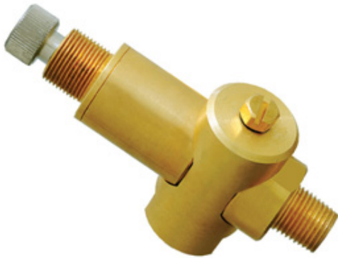
Pressure Regulator, 1/8" NPT Swivel Mount, Knurled Knob, Non-Relieving, 10-20 psig
