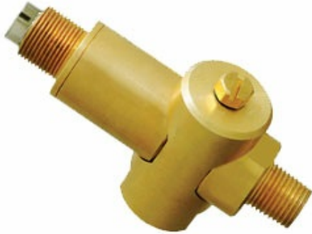
Pressure Regulator, 1/8" NPT Swivel, Screwdriver Slot, Non-Relieving, 10-30 psig
