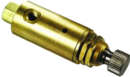
Pressure Regulator, #10-32 Ports, Knurled Knob, 10-40 psig
