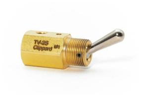
The function of a 2-Way valve is to turn an air supply on and off. In the "on" position, medium flows from the inlet to the outlet, and in the "off" position, the flow is blocked. 3-Way styles have an exhaust port which vents the outlet to the atmosphere. Available with #10-32 and 1/8" NPT ports.
