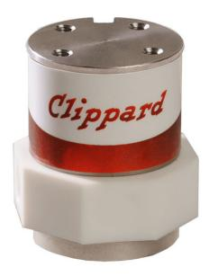
The NIV series media isolation valve is a solenoid-operated device that utilizes a flexible diaphragm to isolate the actuation mechanism from the fluid path. Media isolation valves are commonly used for a wide variety of applications, including those that require precise, repeatable dispensing of media for analytical instrumentation. All wetted areas of the valve are PTFE or PEEK, making this series ideal for use with corrosive media.
