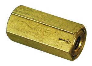
Check valves permit flow in one direction only. The MCV series is available with #10-32 ports and are construced of bright-dipped brass bodies that provide in-line mounting.
