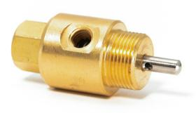
The MAV series are #10-32 ported valves that change their flow path when the stem is depressed or released. The 2-Way and 3-Way valves are offered in both Normally-Closed (not passing) or Normally-Open (passing) versions.
