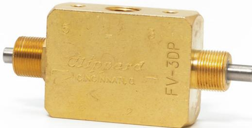
The FV series are #10-32 or 1/8" NPT spool valves which are fully-ported, which means that all ports are usable and can handle pressure or vacuum or both. This series offers Normally-Open, Normally-Closed and Selector/Divertor functions.
