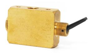
3-Way, 2 Position FTV valves have a supply, outlet and exhaust port. When the toggle is in the "on" position air flows from the inlet to the outlet and the exhaust port is blocked. Moving the toggle to the "off" position closes the inlet and opens the outlet to an exhaust port which vents the outlet to atmosphere. 3-Way toggle valves may have a poppet or spool and by movement of the toggle may either be 2-position or have a momentary actuation.
