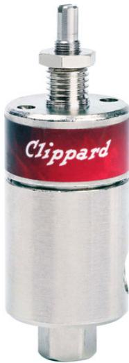
The DR-2 precision regulators are offered in either relieving or non-relieving versions. The relieving design maintains a constant pressure output even when downstream conditions change, while non-relieving regulators do not automatically compensate for changes in downstream flow or pressure. There is no vent to atmosphere, as in a relieving type regulator, and the output pressure can increase due to a downstream event. Non-relieving versions can also accommodate compatible liquid applications.
