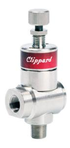
The DR-2 precision regulators are offered in either relieving or non-relieving versions. The relieving design maintains a constant pressure output even when downstream conditions change, while non-relieving regulators do not automatically compensate for changes in downstream flow or pressure. There is no vent to atmosphere, as in a relieving type regulator, and the output pressure can increase due to a downstream event. Non-relieving versions can also accommodate compatible liquid applications.
