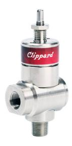
The DR-2 precision regulators are offered in either relieving or non-relieving versions. The relieving design maintains a constant pressure output even when downstream conditions change, while non-relieving regulators do not automatically compensate for changes in downstream flow or pressure. There is no vent to atmosphere, as in a relieving type regulator, and the output pressure can increase due to a downstream event. Non-relieving versions can also accommodate compatible liquid applications.
