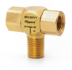
Shuttle valves feature a shuttle that allows flow from one inlet to the outlet while blocking the other inlet. They may be mounted directly to valves or in-line using the hose barbs.
