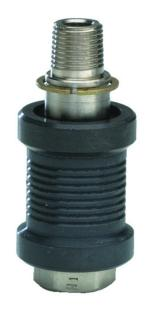
The J-Series sleeve valves with 1/8" NPT and 1/4" NPT ports offer large flow capability with a relatively short stroke in 2-Way and 3-Way valves, and no cross-over between inlet and exhaust on the 3-Way models.
