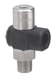
Pilot-operated check valves work as standard check valves but can be opened with an air pilot signal to permit free flow in the normally "checked" direction. This provides the user with a reliable method to check flow in one direction with the ability to remotely signal a free flow through the valve. The JPC Series all-in-one pilot-operated check valves are easy to connect and ideal for any circuit that might benefit from this useful function.
