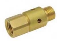
J-Series Exhaust Valves offer a variety of design features and provide fast response times and high flow with 1/8" and 1/4" NPT ports. This compact poppet type valve is constructed of brass and is 100% tested to assure the highest quality.
