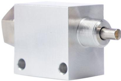
The MJV/MJVO series are high flow 1/8" NPT ported 2-Way, 3-Way and 4-Way valves that change their flow path when the stem is either depressed or released (spring return). The 2-Way and 3-Way valves are offered in both Normally-Closed and Normally-Open versions.
