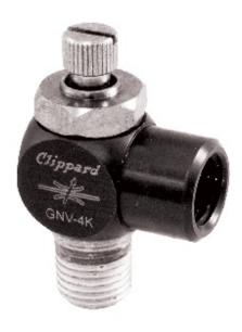
Needle Valves are used to control the rate of flow in a pneumatic system by controlling flow in both directions. Material enters the input port, travels through an adjustable orifice and out the output port.
