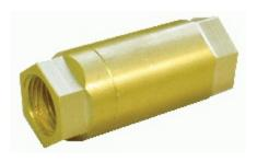
Check Valves permit flow in one direction only. Each has bright-dipped brass bodies that provide in-line mounting, Nitrile seals and stainless steel springs as standard. Available in 1/8" NPT, G1/8, 3/8" NPT and G3/8 ports.
