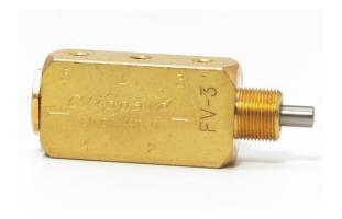
The FV series are #10-32 or 1/8" NPT spool valves which are fully-ported, which means that all ports are usable and can handle pressure or vacuum or both. This series offers Normally-Open, Normally-Closed and Selector/Diverter functions.
