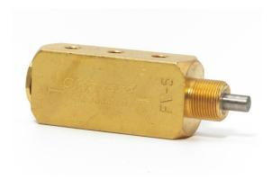
The FV series are #10-32 or 1/8" NPT spool valves which are fully-ported, which means that all ports are usable and can handle pressure or vacuum or both. This series offers Normally-Open, Normally-Closed and Selector/Diverter functions.
