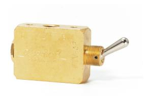
3-Way, 2 Position FTV valves have a supply, outlet and exhaust port. When the toggle is in the "on" position air flows from the inlet to the outlet and the exhaust port is blocked. Moving the toggle to the "off" position closes the inlet and opens the outlet to an exhaust port which vents the outlet to atmosphere. 3-Way toggle valves may have a poppet or spool and by movement of the toggle may either be 2-position or have a momentary actuation.
