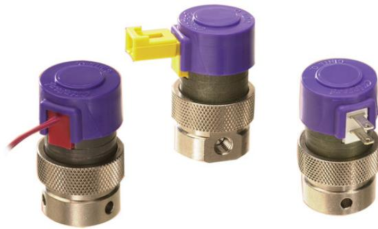
The EVP 2-Way proportional control valves combine the features of the existing EV series valve—long life, low power, and Clippard's reputation for high quality components—with the additional capability for proportional control. The EVP series valve provides air or gas flow control, and varies the output flow based on the current input to the solenoid.
