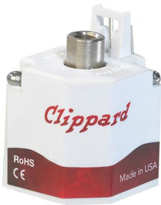
The ES series features large cross sectional o-rings, minimal leak points, and proven poppet designs. All mounting hardware is outside of the flow path for the ES, and no internal parts are threaded during assembly to reduce the possibility of contamination. The ES has the best performance-to-price ratio for low leak valves.
