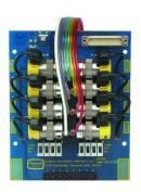
Direct low voltage DC signals from controllers, systems, computers or other sources to operate powerful pneumatic valves with a minimum of piping and hook-up. Cards contain 8 or 12 Clippard ET electronic Valves; fully-wired circuit board; plug-in with 25-pin connector, resistor, diode, LED and switch for each valve; and auxiliary power supply connection.
