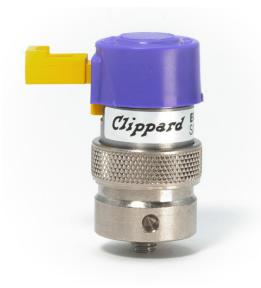
The EVP 2-Way proportional control valves combine the features of the existing EV series valve—long life, low power, and Clippard's reputation for high quality components—with the additional capability for proportional control. The EVP series valve provides air or gas flow control, and varies the output flow based on the current input to the solenoid.
