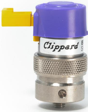
The EVP 2-Way proportional control valves combine the features of the existing EV series valve—long life, low power, and Clippard's reputation for high quality components—with the additional capability for proportional control. The EVP series valve provides air or gas flow control, and varies the output flow based on the current input to the solenoid.
