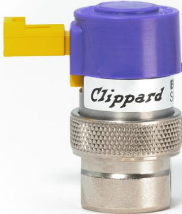
The EVP 2-Way proportional control valves combine the features of the existing EV series valve—long life, low power, and Clippard's reputation for high quality components—with the additional capability for proportional control. The EVP series valve provides air or gas flow control, and varies the output flow based on the current input to the solenoid.
