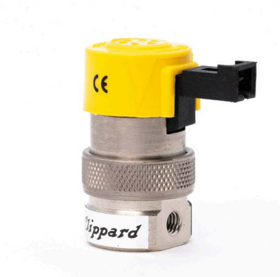
2-Way Elec. Valve, N-C, In-Line Mount, Pin Connector, 24 VDC
