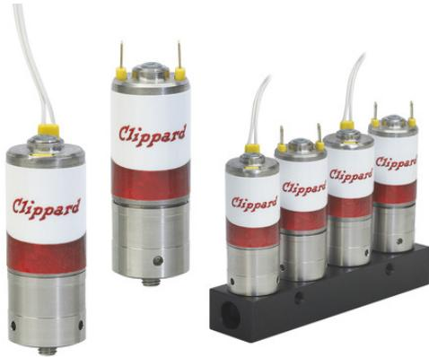
The DVP Series proportional solenoid valves are precision-built 2-way control valves, utilizing a unique, patented valving principle. They offer an extremely high cycle life, fast response, linear flow gain, low hysteresis, low power consumption, and flows over 60 l/min. The valve provides air or gas flow control, and varies the output flow based on the current input to the solenoid.
