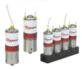
The DVP Series proportional solenoid valves are precision-built 2-way control valves, utilizing a unique, patented valving principle. They offer an extremely high cycle life, fast response, linear flow gain, low hysteresis, low power consumption, and flows over 60 l/min. The valve provides air or gas flow control, and varies the output flow based on the current input to the solenoid.
