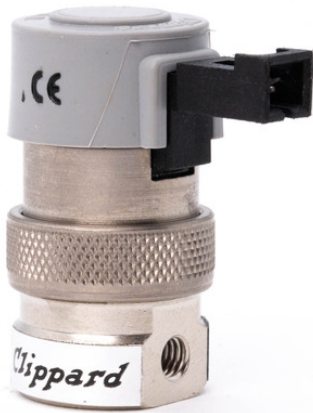
3-Way Elec. Valve, N-C, In-Line Mount, Pin Connector, 12 VDC
