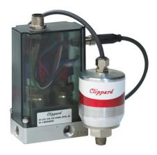
Clippard CPS series pressure sensors are conditioned and offer a customized calibration around your application requirements, allowing for a full scale accuracy of 0.25% over the calibrated range. They can be used in conjunction with Clippard's Cordis Pressure Controller or as a standalone transducer.
