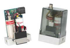
The Cordis Flow Controller utilizes an extremely fast-reacting MEMS technology sensor upstream from Clippard's proportional valve. Unlike other mass flow controllers, the Cordis flow controller requires less than one minute warm-up, features a pressure drop ≤14" H2O, and includes flow ranges as low as 0 to 30 sccm. Standard control options include 0.2 to 10 VDC, 4.32 to 20 mA, and 3.3 VDC Serial. IP65 housing available for light industrial applications.
