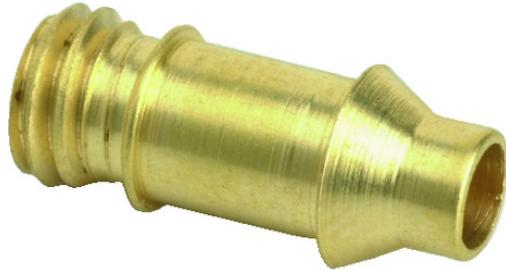
Minimatic barb fittings provide a flexible, easy alternative to ferrule and push-to-connect/push-quick fittings. Designed for use with urethane hose, barb fittings will provide a leak-free connection that will hold well beyond the working pressure of the hose without the need for additional clamps.
