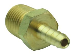
Minimatic barb fittings provide a flexile, easy alternative to ferrule and push-to-connect/push-quick fittings. Designed for use with urethane hose, barb fittings will provide a leak-free connection that will hold well behond the working pressure of the hose without the need for additional clamps.
