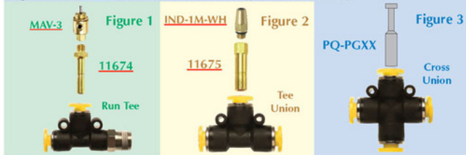
Figure 1 shows an MAV-3 3-Way Valve connected to a PO-RT05P Run Tee using a 11674-05 Adapter. In this example, the Run Tee is connected to a 1/8" NPT supply pipe. Figure 2 shows an IND-1M-WH Pressure Indicator connected to a PQ-TU08 Tee Union using a 11675-08 Adapter. If one of the branches of a Push-Quick Fitting is to be used as a temporary pressure gauge port, the PQ-PGXX series of Plugs can be used when the gauge is not in place. Plugs may also be used if Push-Quick Fitting branches are intended for future additions to the circuit, but have no current need. Figure 3 shows a PQ-CU Cross Union with one branch plugged with a PQ-PG08 Plug.
