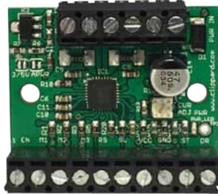
**RST (Reset):** This input is tied high with a 20K Ohm resistor on the driver. If this signal is pulled low, the motor driver circuits are shut off and the driver is reset. Only when this input is high will the driver chip enable the motor driver circuits and react to the step input.
