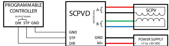
This diagram illustrates a typical connection (the bare minimum connection) for the SCPVD-1 with a Clippard SCPV valve and a source for step/direction signals. Additional digital input signals may be connected on the SCPVD-1 for more control (Sleep, MS1, etc.). A typical setup will have MS1, MS2, and MS3 set low (connected to ground) for full stepping mode.
