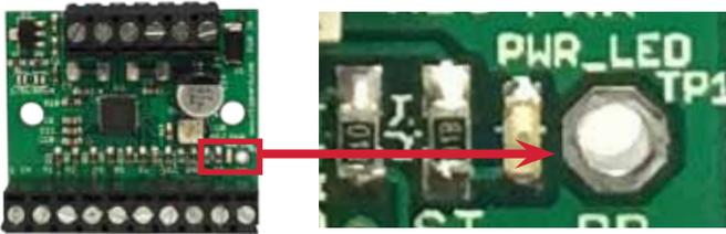
A volt meter is used to measure the voltage on TP1 (Vref) with respect to GND as the potentiometer is turned.
