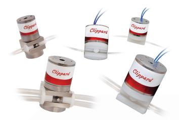
NPV series pinch valves are solenoid-operated devices that are designed to open and close tubes for controlling flow of liquids and gases. Whereas other valve types have internal passages that may cause small amounts of fluid to remain in the valve, pinch valves have no areas where fluid can become trapped. Energizing the solenoid retracts or attracts the plunger, which opens or closes the tube, while de-energizing the solenoid allows the plunger to return to its original state.
