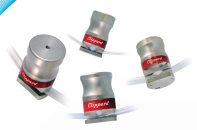
Clippard's NPP series pinch valves utilize an air-piloted design to provide the same functionality and benefits as the NPV series but with the added benefit of lower power and greater force. This makes them ideal for applications that are particularly sensitive to heat or those that require larger or firmer tubes.
