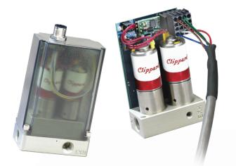
The Cordis CPC is a closed-loop pressure control valve system designed to maintain a steady and repeatable downstream pressure as demand or process changes occur. It is available in a compact card style (CPC-C) or with an IP65 rated enclosure (CPC-H) for manufacturing and industrial environments, and is also available in a CE-approved version. All styles come standard with two Clippard proportional electronic valves designed for high resolution pressure control.
