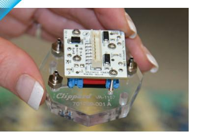
Value-added sub-assembly with custom acrylic manifold
