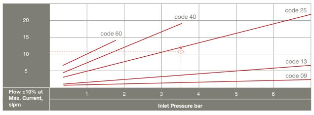
To determine the correct orifice code, locate the red line immediately above the flow/pressure intersection. Example: 11 slpm @ 3.5 bar inlet, aquires the orifice code 25 for your part numbering system at following two pages. Based on Clippard's original spider design from 1973, the EVP's armature is the heart of the valve which provides precise flow control.
