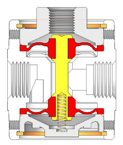
providing the same assurance of return to a given position as the poppet valve. The diaphragm increases durability especially with different or non-lubricated media. The diaphragm also allows for the potential use of liquids through the body of the valve depending on application and rubber compatibility. A variety of durometer and diaphragm compounds make it simple to modify a valve based on the environmental or application requirements for operation. Also,
