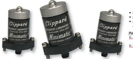
The **R-337** is a 3-way, spring return, fully-ported, piloted valve with an independent check valve in the same body. It can be used Normally-Open, Normally-Closed, as a diverter or as a selector.
