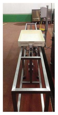
Charter Engineering Group was contracted by a Northwest US-based food manufacturer to design and fabricate a machine to automate a manual fill operation. The fill material is a heated, viscous cheese product that is poured into fiberglass trays and later cooled and cut for packaging. Clippard Minimatic supplied the pneumatic components used in the design.
