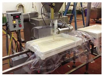
In this application, the trays are filled with product to a customer-selected weight (typically 40 to 100 lb) while air cylinders and pneumatic logic control the index movements.
