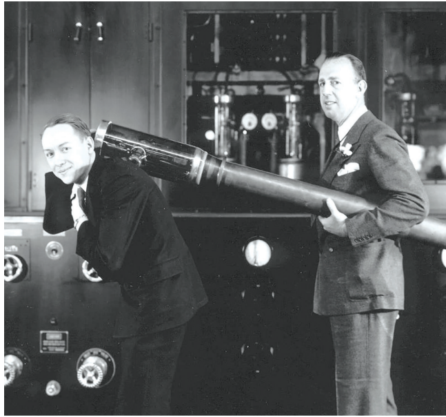
May, 1934 - Powel Crosley, Jr. (right) and Joseph Chambers, WLW Technical Supervisor, "hefting" one of the twenty huge 100,000 watt tubes used in the new 500,000 watt WLW Transmitter
